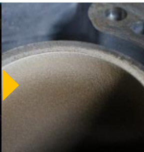
Cylinder after coating
