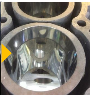
Cylinder after final machining (Mirror honing)
