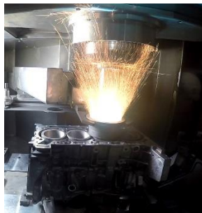
Molten metal sprayed by a rotating nozzle
